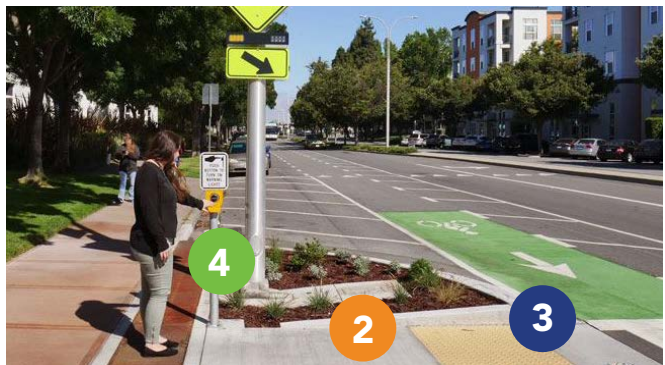
Midblock crossing with beacons and signals
