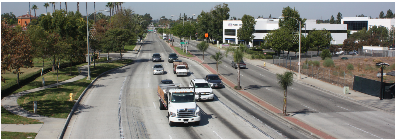
Roadway noise is the collective sound energy emanating from motor vehicles, consisting primarily of road surface, tire, engine/transmission, aerodynamic, and braking elements. Noise of rolling tires driving on pavement is found to be the biggest contributor of roadway noise and increases with higher vehicle speeds.
