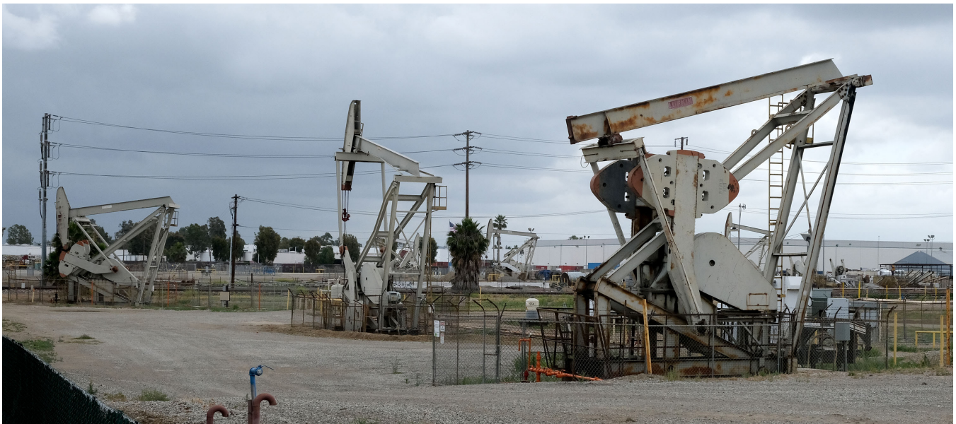
Oil derrick pumps continue to pull oil from underground wells up to the surface within the Santa Fe Springs oil field.
